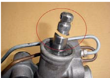
Arbore deteriorat sau rupt
