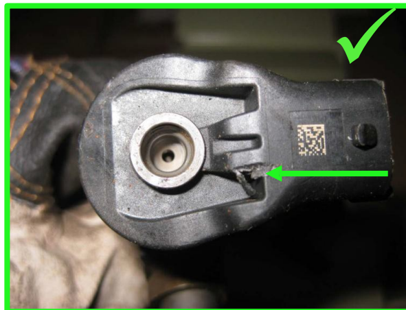
Carcasa electromagnet deteriorata → acceptabil
