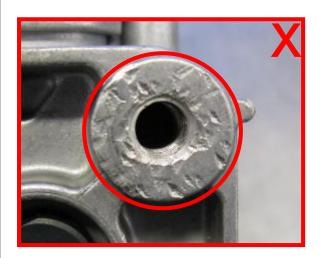
damage on thread  $\rightarrow$  not acceptable
