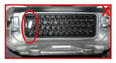
pins deformed / corroded → not acceptable
