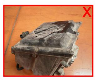
damage on housing cap → not acceptable
