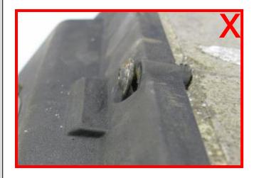
aggregate was opened / screws are loose / screws are missing
